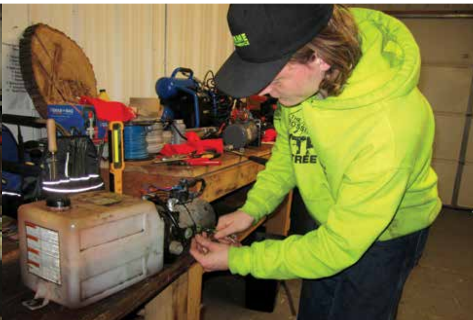
Andi Campos, 19, (left) demonstrates equipment used by Crossing students in training at Thor Motor Coach. Darren Maddox, 18, repairing a hydraulic pump for a truck, helps keep equipment running smoothly for the student-run Xtreme Tree Service business.
