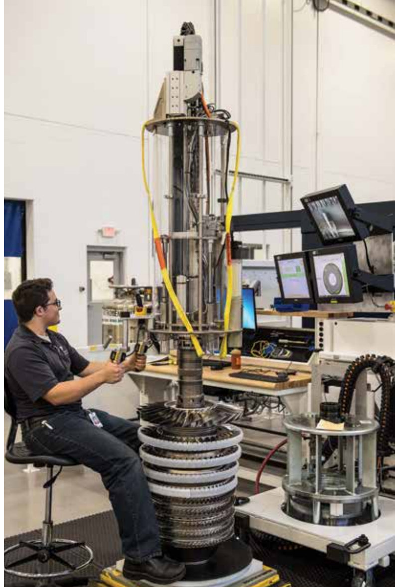
A LEAP 1A (for the Airbus A320neo family of aircraft) compressor joint is being torqued by an automatic wrench that was designed by GE technicians. The joint cannot be reached by traditional tools.
