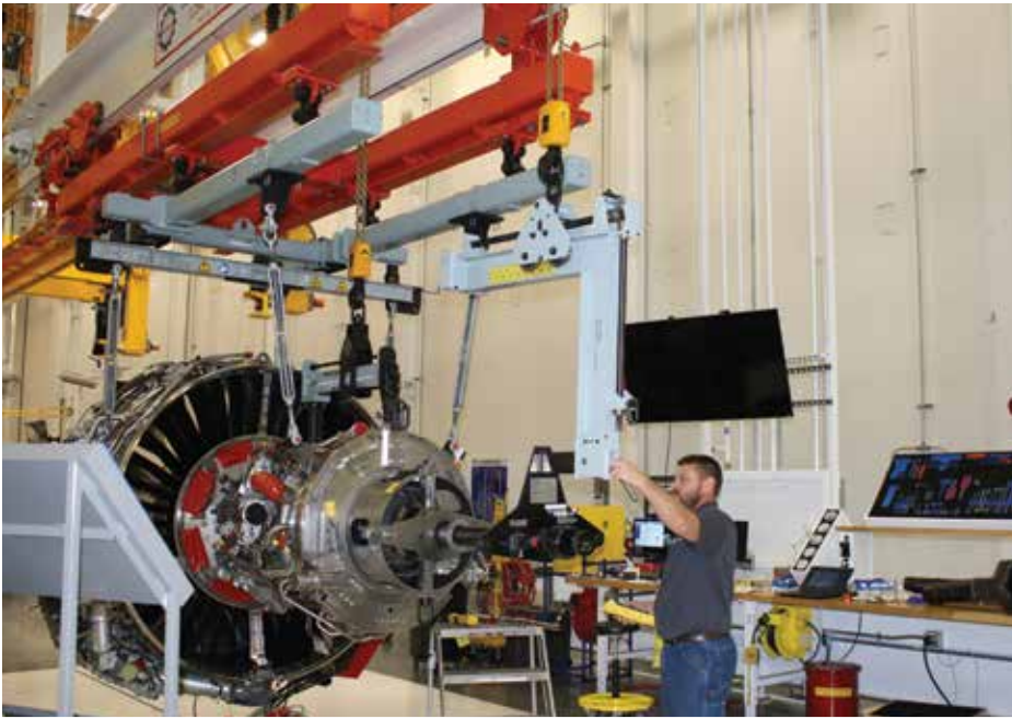
The LEAP 1B (for the Boeing 737 MAX) core is mated to the fan in final assembly (top). Stage 2 nozzle sub-assembly is a 12-hour process that grinds all of the assembled parts in the module to specific tolerances.
