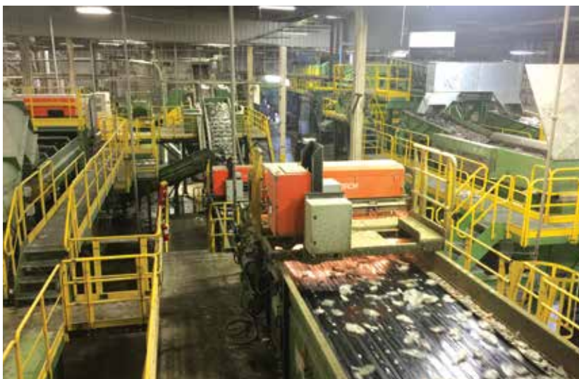
Bottles travel through a sorting line at Perpetual Recycling Solutions. An East-Terra Plastics team member inspects material before it’s loaded into a grinder.
