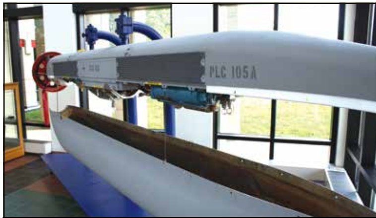
Outdated weaponry and war relics can be found displayed around Crane. This tactical jamming System Pod was flown on the EA-6B and EA-18G aircrafts and was used to suppress enemy radar systems.
